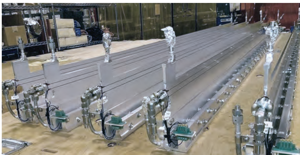
Fig. 2. Five HXR chambers assembled in alignment fixtures, with water fittings and Earth-field coils. Photo by Dave Boughton
