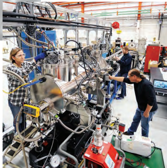
Above: Technicians from the APS Accelerator Systems Division Magnetic Devices Group and the APS Engineering Support Division Survey and Alignment Group working on a helical superconducting undulator insertion device. Super-conducting undulators are now in operation in the APS storage ring and are a key component of the APS-U. They produce stronger magnetic fields and thus higher-energy x-rays than conventional permanent magnetic undulators having the same period lengths.
