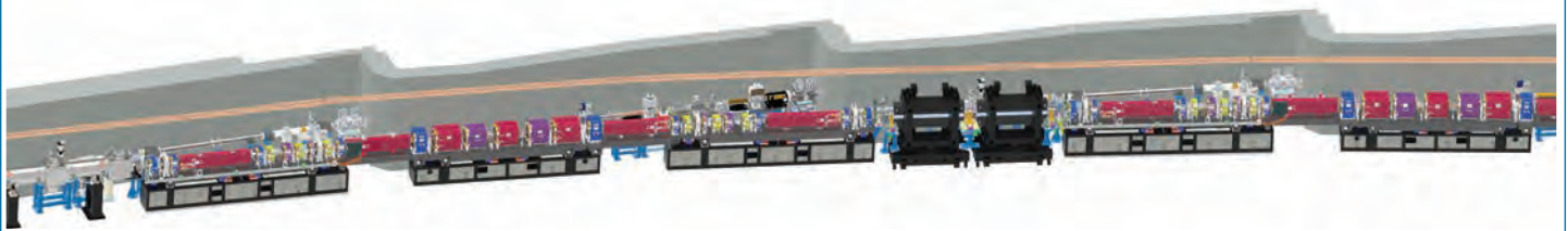
Above: A computer-aided rendering of a typical APS-U storage ring sector showing the MBA-lattice configuration of red, blue, and purple electromagnets and associated components. Rendering by the AES Design and Drafting Group.
